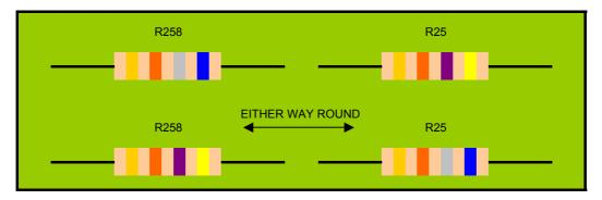
Check resistors R25 and R258 on the outdoor PCB.
